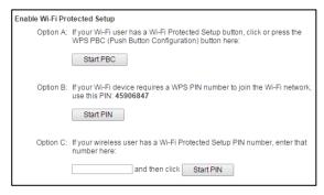
**Option A:** Push button: You may push the WPS button on the web menu or use the physical button on the back of the Router.
