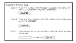
**Option A:** Push button: You may push the WPS button on the web menu or use the physical button on the back of the Router.
