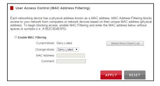
A MAC Address may sometimes be referred to as a Physical Address. Most networking devices have their MAC Address located on a label on the actual device.
